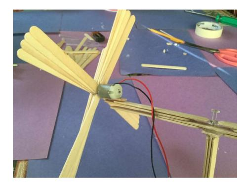
17. Get five sticks and glue them on top of one another as if placing them into a stack. Then glue the stack on the side that has the triangular tail. This is done in order to balance the weight of the blades and tail.
