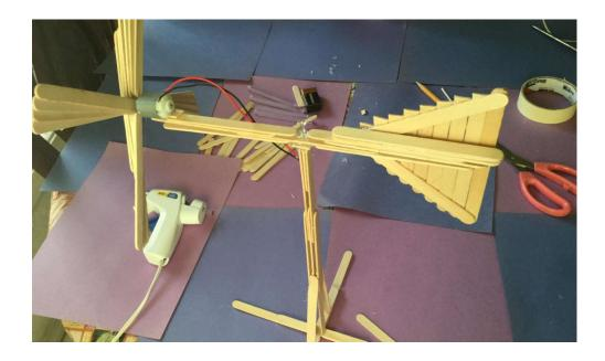
18. Make sure that your base is not tilting back and forth and that the weight is well-balanced. Finally, glue the 9V battery at any convenient space. The wires of the DC motor should be able to connect to the battery.
