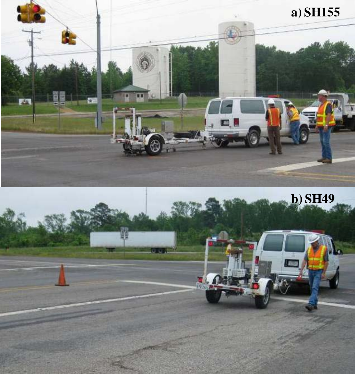
Figure 5.8 - FWD Collection on SH 155 and SH 49 Images.
