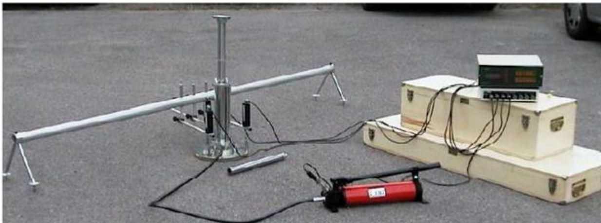
Figure 2.8—Plate Bearing Test Apparatus
