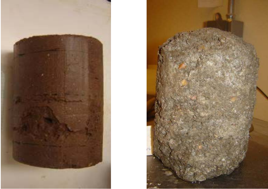
Figure 4.8 – Submerge Test Specimens after Test
