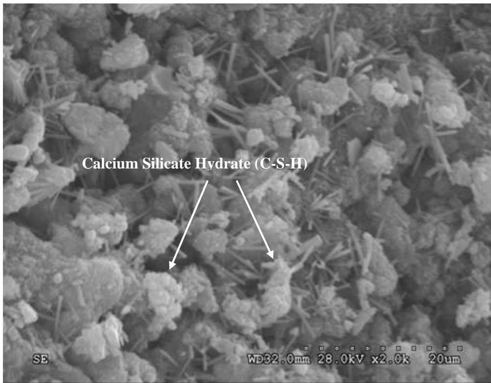
Figure 5.17 – Typical SEM Image for 75R_2C Mix (Powered) from El Paso District
