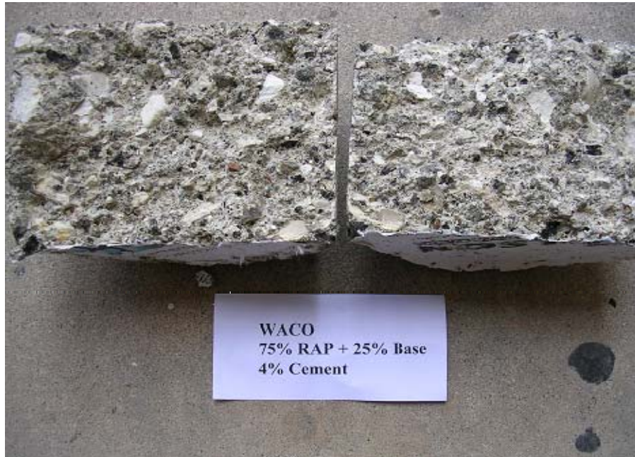
Figure 4.20 – Breaking of Virgin Base Aggregate in RAP Blend from Waco District
