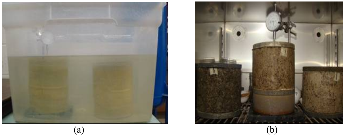
Figure 5.1 – Test Setup for Wetting/Drying Process: (a) Wetting, (b) Drying
