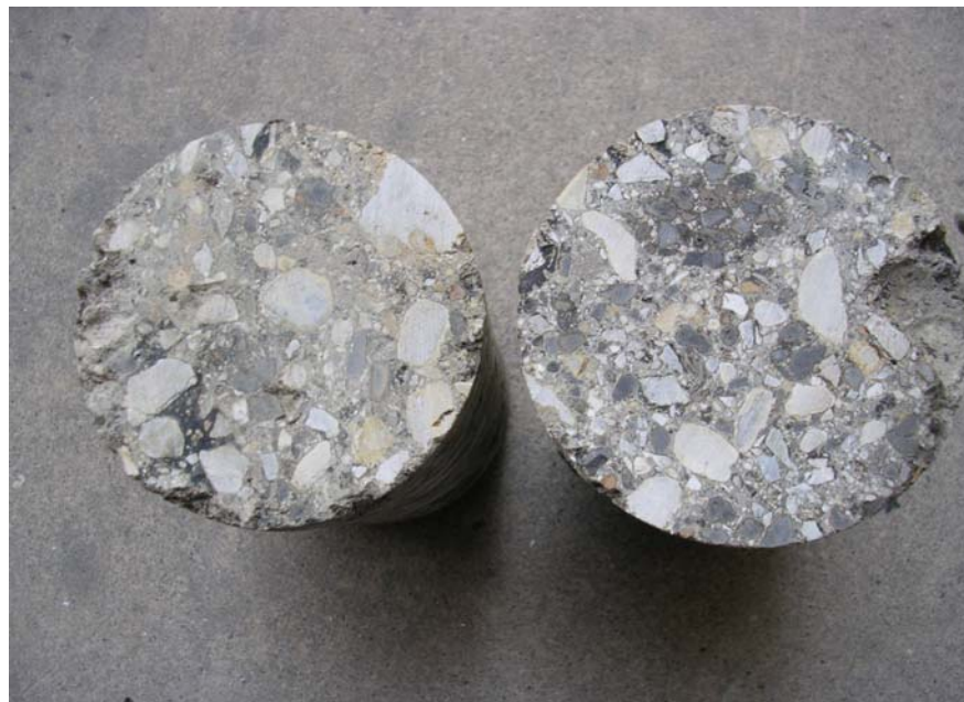
Figure 6.16 – Cores Retrieved from New Base of the FM 2415 Project
