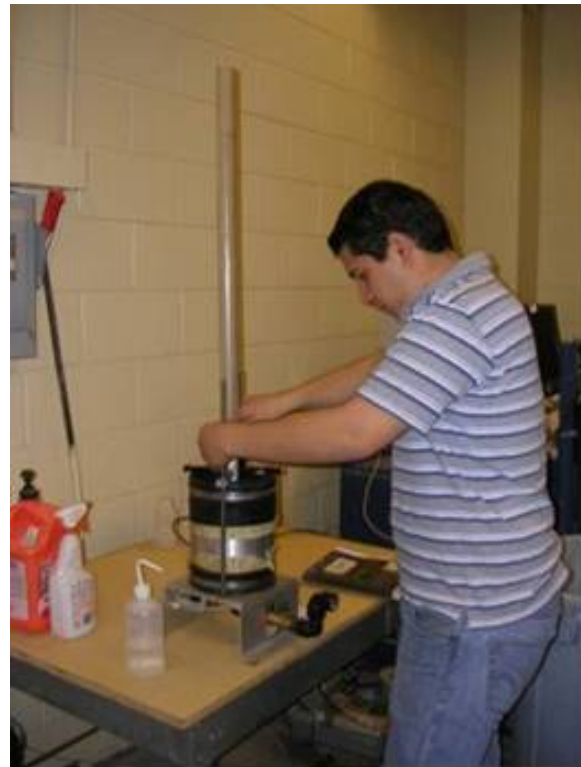
Figure 4.3 – Setup for Hydraulic Conductivity Test
