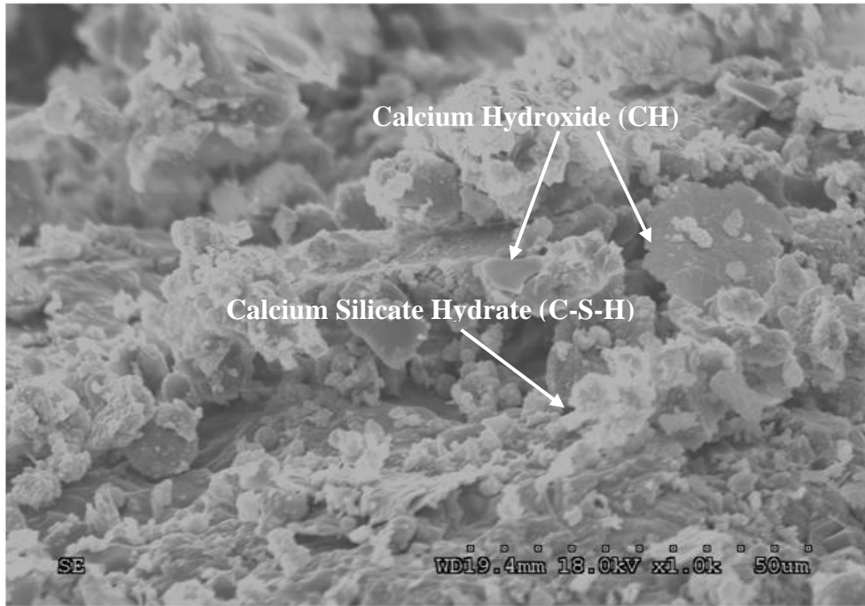
Figure 5.14 – Typical SEM Image for 100R_6C Mix (Powered) from El Paso District
