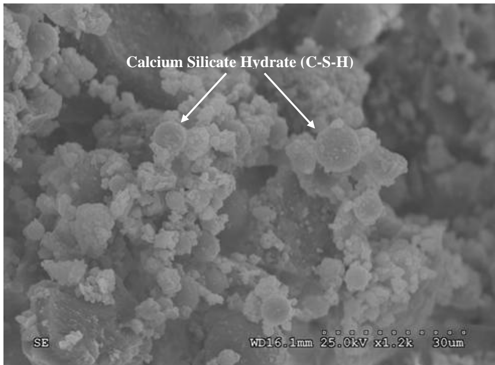
Figure 5.16 – Typical SEM Image for 60R_2C Mix (Powered) from El Paso District
