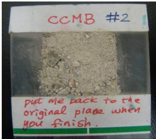
Figure 5.6 – Sample Holder with Typical Powdered RAP Mix
