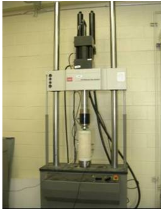
Figure 4.1 – Equipment and Setup for Resilient Modulus and Permanent Deformation Tests
