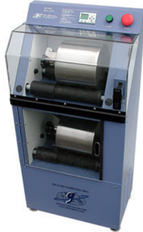
Figure 5.14 - Micro-Deval Machine (Gilson Company website)
