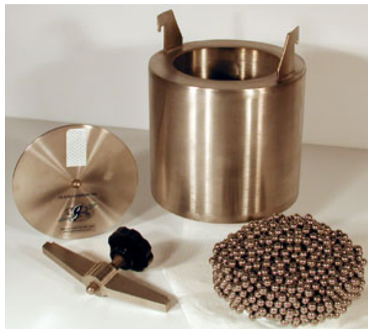
Figure 5.13 - Micro-Deval jar and Steel Balls (Gilson Company website)
