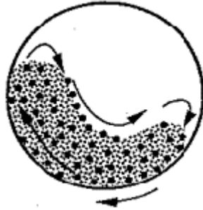
Figure 5.12 - Interaction between Aggregates and Steel Balls in Micro-Deval
