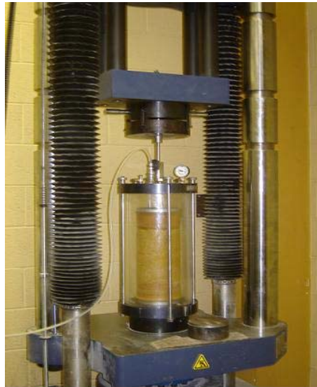
Figure 7.3 - Schematic of Triaxial Compressive Tests
