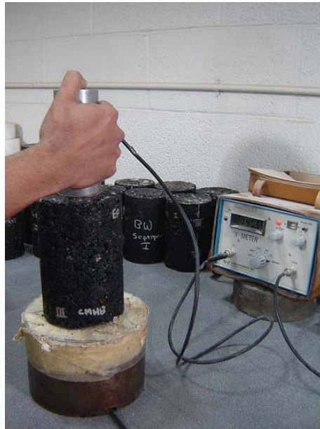
Figure 6.7 - V-Meter Test Set up
