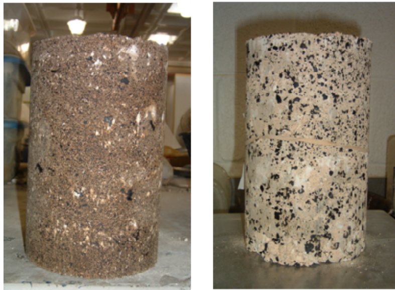
Figure 5.8 – Appearances of Specimens Mixed with High-Shear Mixer (left) and Concrete Mixer (right)
