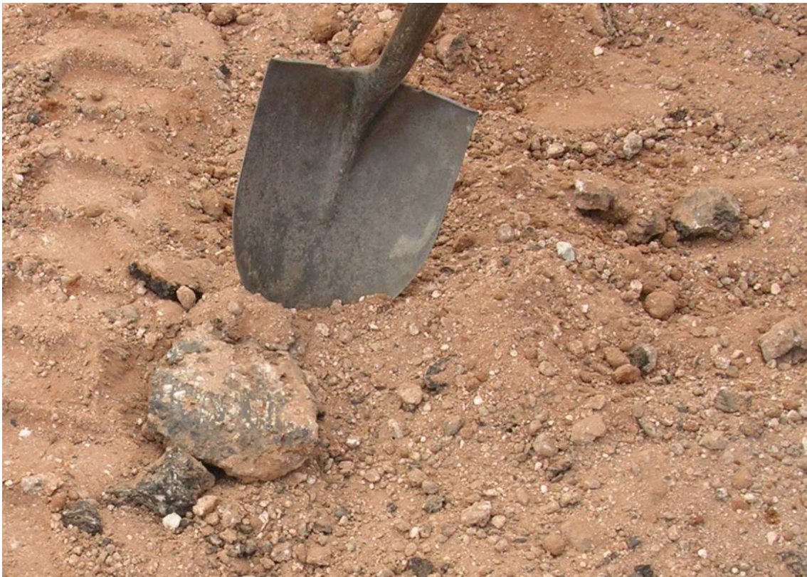
Figure 5.7 - Large-size HMA after pulverization
