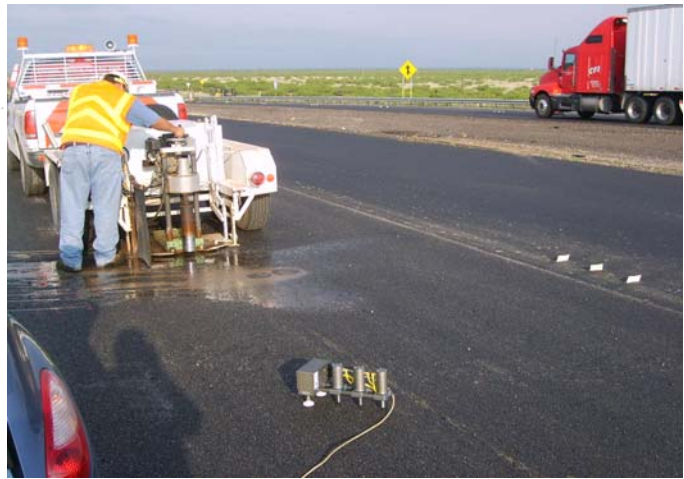
b) Coring and PSPA Testing
