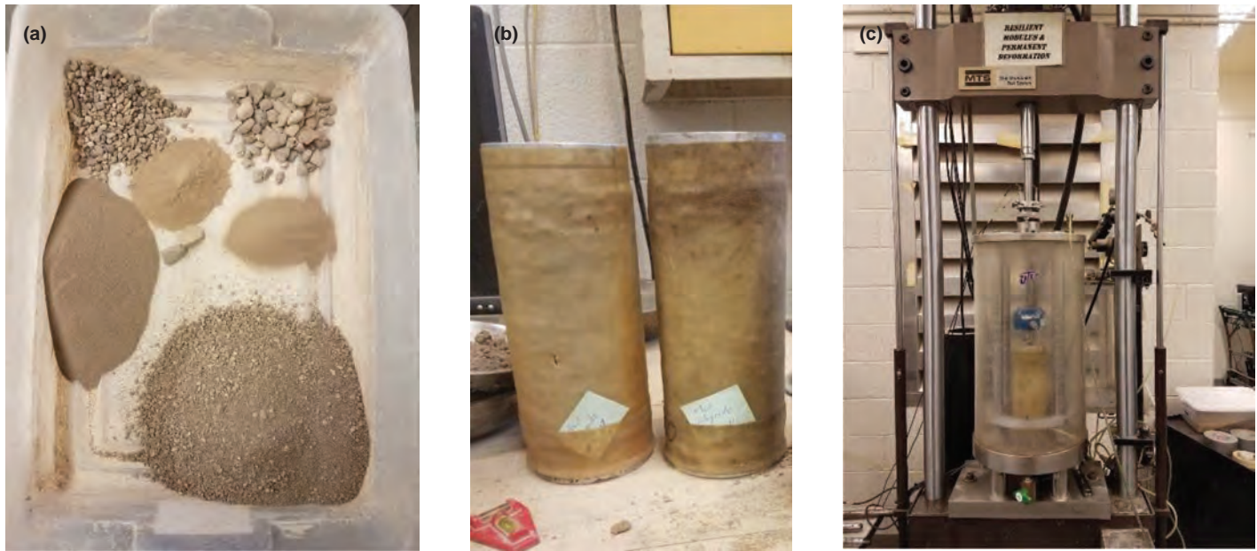
Figure 7-9. Preparation of soil for testing: (a) soil mixture based on the sieving analysis, (b) prepared samples for resilient modulus test, and (c) MTS® Load Unit System.
