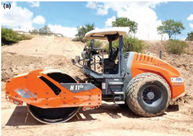
Figure 7-8. Smooth-drum IC rollers used for mapping: (a) Hamm H 11ix, used at Site 1, and (b) Caterpillar CS74B, used at Site 2 and Site 3.
