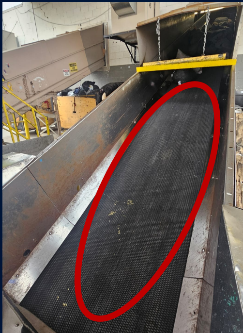
4. Infeed conveyor inefficient utilization
