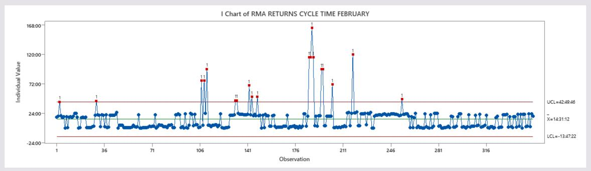
Above is an Individual Chart of the RMA Returns Cycle Time from February, displaying a mean of x = 14:31:12, from each of the individual observations. The upper and lower control limits are also shown, and we see how many of the data points are out of control by them surpassing the upper control limit of 42:49:46
