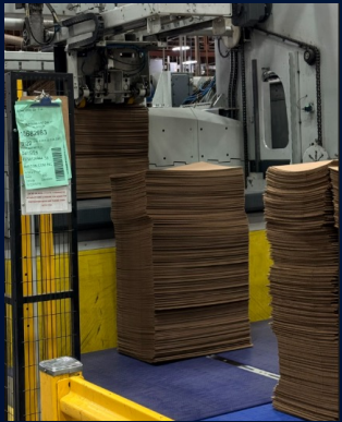
Corrugated Boards are loaded on to the Prefeeder
