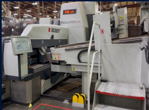
Prefeeder extends corrugated boards and loads them on to the print section
