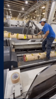
Die Cut Section makes insertions to corrugated board
