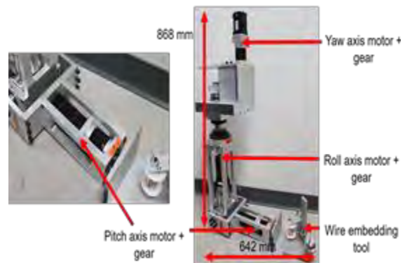
Figure 3: Wire Embedder and the Arm assembled together
