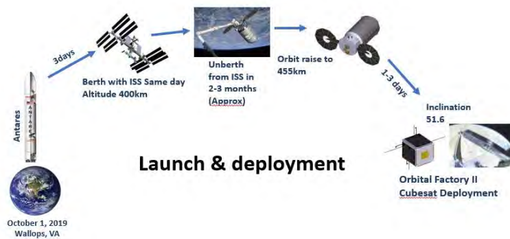
Fig. 1 Launch and deployment of OF-II.
