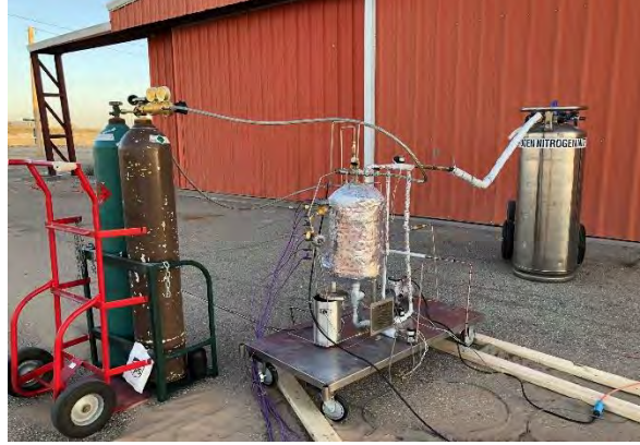
Figure 2: Methane Condensing Unit
