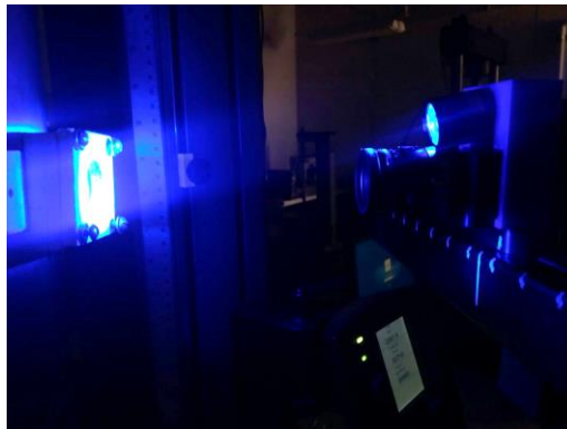
Fig. 2. High temperature DIC setup showing the 2.0 Megapixel Digital Camera and the blue light emitting diode, directly aligned with the specimen through the view port of the split tube furnace.
