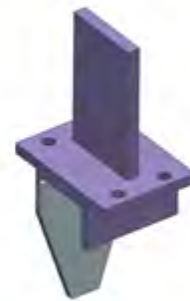
Fig. 4. CAD model of piezoelectric sensor mount.
