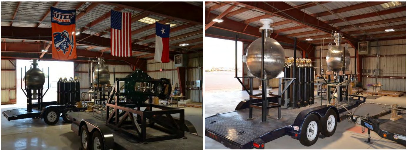
Figure 1. D1 horizontal test facility assembly. a) Isometric image of both trailers in its testing position. b) Image of the propellant trailer which show the run tanks, the pressurant k-bottles and the oxygen run line.
