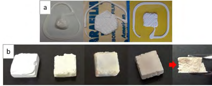
Figure 1. (a) 3D printed samples at different ratios of PVDF-DMF (from left, 1:14 (triangle), 1:10 (hexahedron), 1:8.8 (square)) (b) sintered samples (from left, 1100, 1200, 1300, 1400 °C, and cross-sectional area of the sample sintered at 1400 °C)
