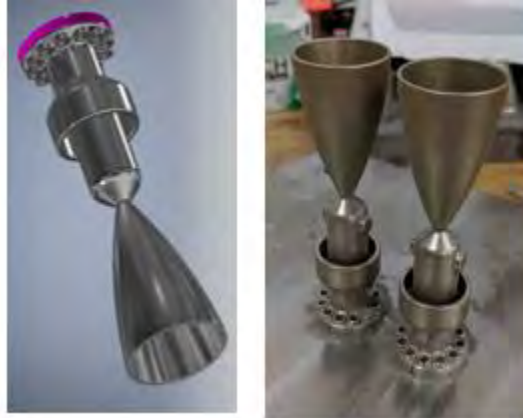
Figure 4: 5N Monopropellant Thrusters Printed with IN 718
