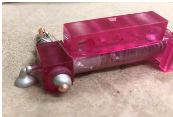
Figure 2: Nozzle failure of previous design iteration
