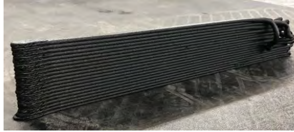
Fig. 2. A single-bead wall printed with an added standby time between layer depositions such that the temperature of the substrate cooled down to approximately 197 °C prior to the deposition of a new layer. Notice the misaligned start of print, and how the deposition is corrected along the direction of deposition.
