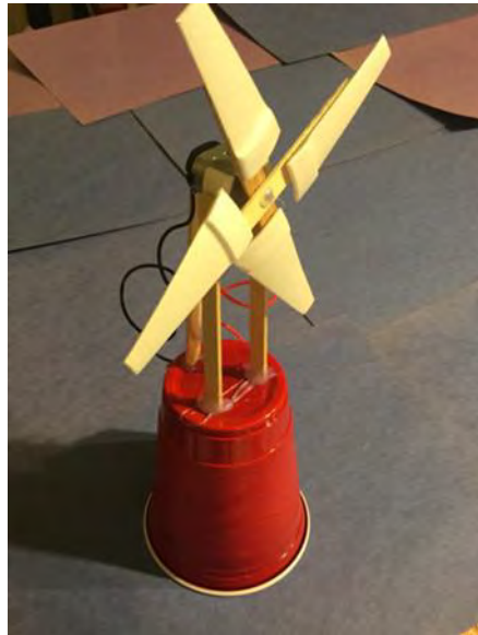
Figure 2: DC Motor-Powered Fan
