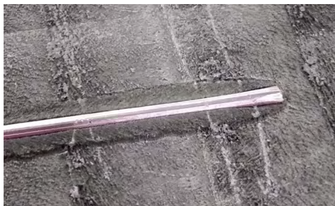
Fig. 1: Embedded wire into a BAAM printed part
