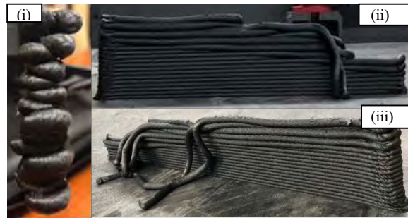
Fig. 3. A single bead wall print with an added standby time between layer depositions such that the temperature of the substrate cooled down to approximately 220 °C prior to the deposition of a new layer. The initial failure occurred at the start of deposition of layer 7.
