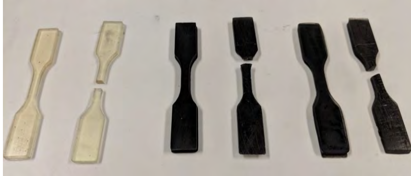
Figure 3. Dog bone samples from left to right Genesis, CNT Functionalized, CNT Functionalized Aligned
