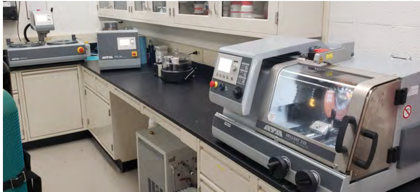
Fig. 5 ATM metallography sample preparation equipment featuring Brilliant 220 precision section saw, vacuum impregnation cold mount station, Opal 460 hot mounting press, and Saphir 530 automated polisher
