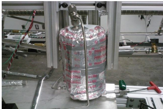
Fig. 2. Tank heat exchanger.
