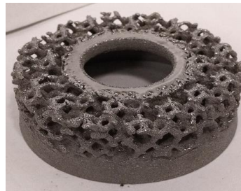
Figure 2. EBM Fabricated parts. Half SRF cavity with lattice structure (Left) and substrate with various complex parts (Right)
