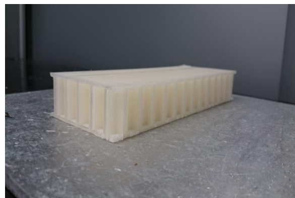
Fig. 5. Normal NX Truss structure after being 3D printed
