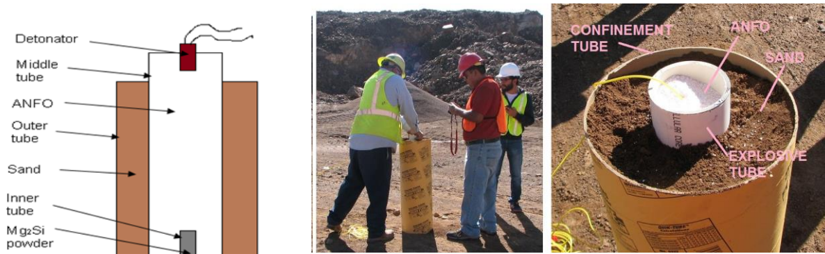
Fig.1. Shockwave consolidation setup.
