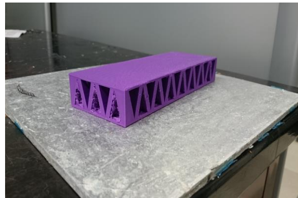
Fig. 3. Diagonal truss design after being 3D printed
