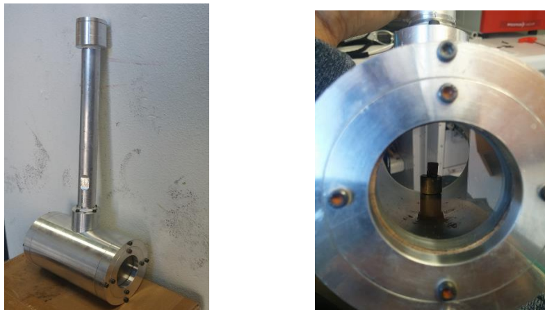
Fig. 1. Chamber for combustion of iodine-generating mixtures.
