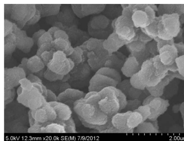
Fig. 2 (a) Scanning electron microscope (SEM) image CoPc-BPDA COF powder.
