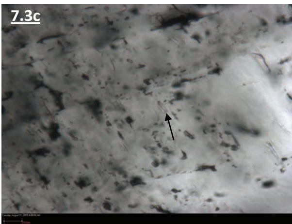
Figure 7.3 Primary fluid inclusions that make up analyzed FIA's within cores from south-central Kentucky. (Figure 7.3a) A FIA composed of four elongate inclusions that are elongate towards the direction of crystal growth from C-295-3. (Figure 7.3b) Three primary inclusions are elongate towards the direction of crystal growth within matrix dolomite from C-511-1. (Figure 7.3c) A set of three two-phase inclusions hosted within the outer portion of a late-stage saddle dolomite cement. (Figure 7.3d) Three two-phase inclusions within a late-stage rhombic dolomite cement.
