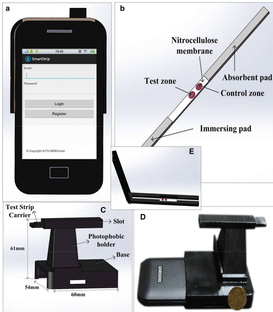
Figure 1. Different views of SmartStrip system. (a) A front view of SmartStrip system. (b) An overview of test strip. (c) A schematic diagram of the smartphone accessory. (d) A picture of the SmartStrip system. (e) A schematic diagram of test strip carrier.
