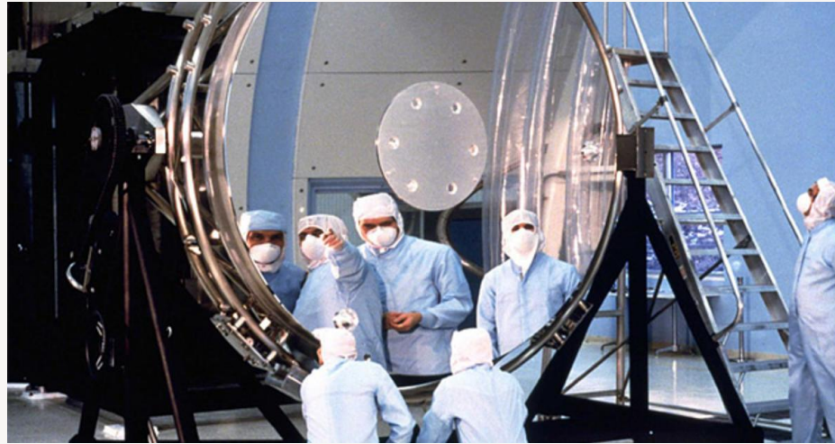
Circular lens mirror used in the Hubble space telescope
