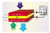
**Project Description:** Novel functional materials that can operate as fuel-cell electrolytes at intermediate temperatures (within the 150°C - 500°C range) are of particular importance for large scale clean-energy applications (e.g. in the automotive industry), as well as for more specific applications based on the
